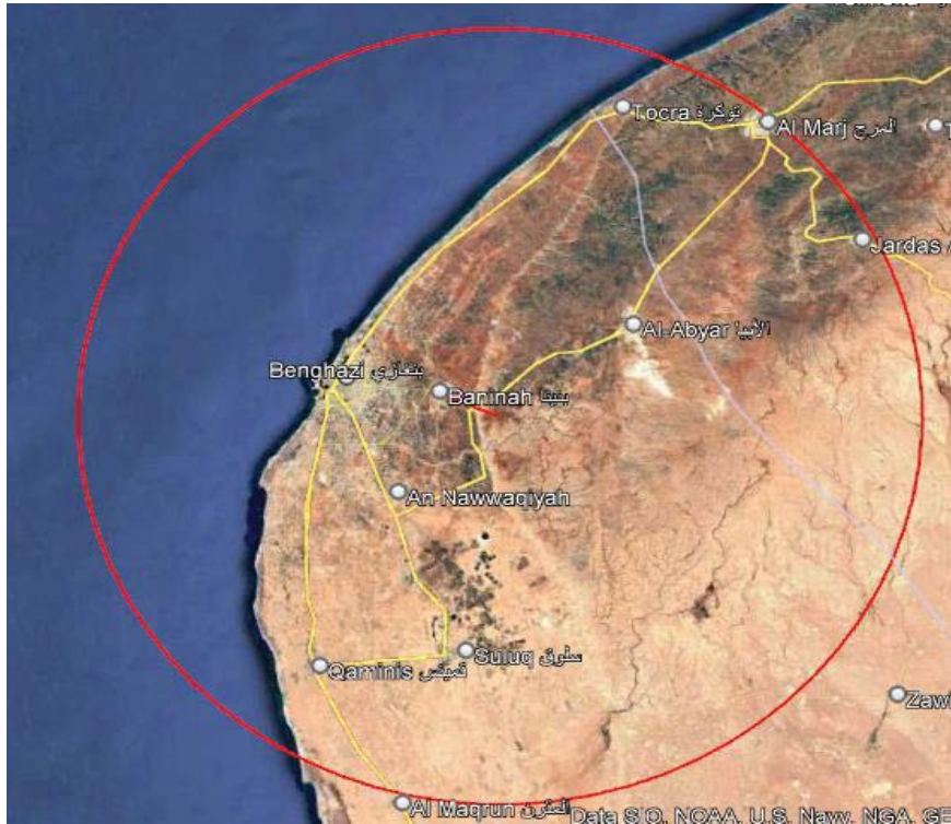
Figure 1 shows the coverage area of Benghazi city. Having one HAPS we designed the altitude of it 25Km to cover area until AL-Marj city from the east, to Al Maqrun from the west.
