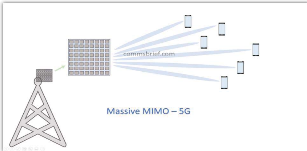
Figure 1 5G Massive MIMO technology .
