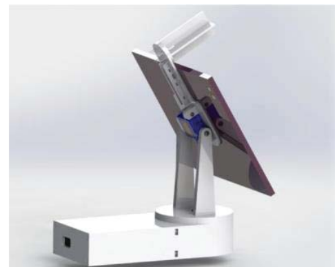
Figure (5) Engineering design of: a) the base of the dual-axis solar tracker, b) vertical axis of a dual-axis solar tracker, c) horizontal axis of a dual-axis solar tracking device
